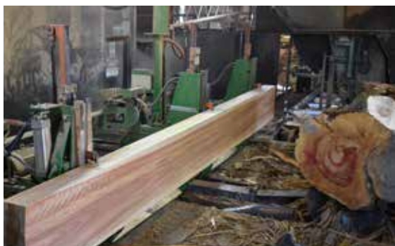
A freshly sawn tōtara beam being milled into planks, showing attractive heartwood.
