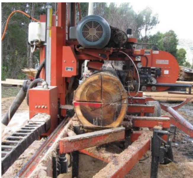
Left: A Wood-Mizer band sawmill in action quartering a pruned blackwood log. Right: A large pruned macrocarpa log being sawn with a Wood-Mizer. Photos: Paul Millen
