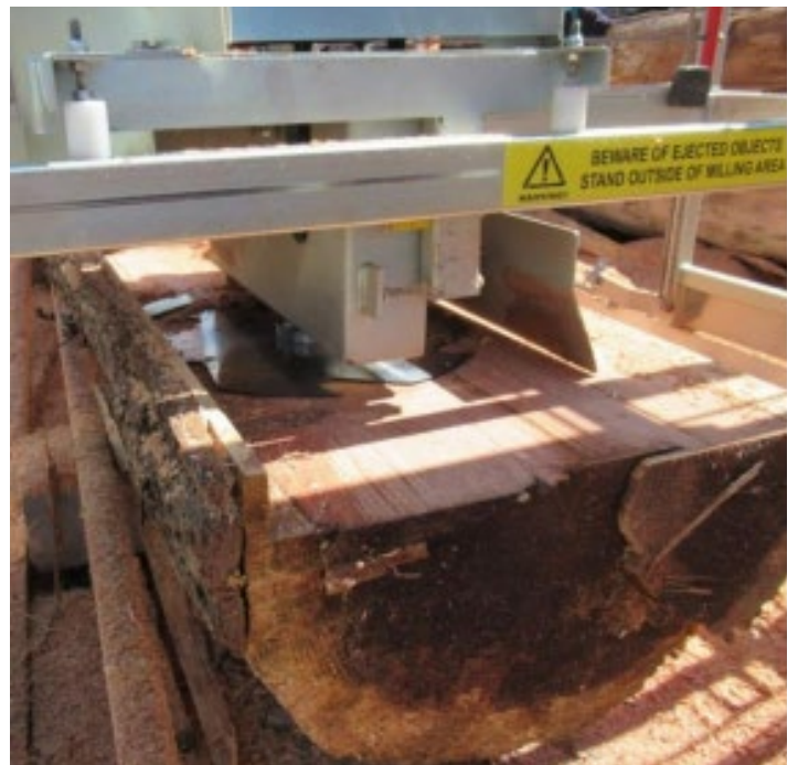
The swing blade circular saw in horizontal cutting position. Photo: Paul Millen
