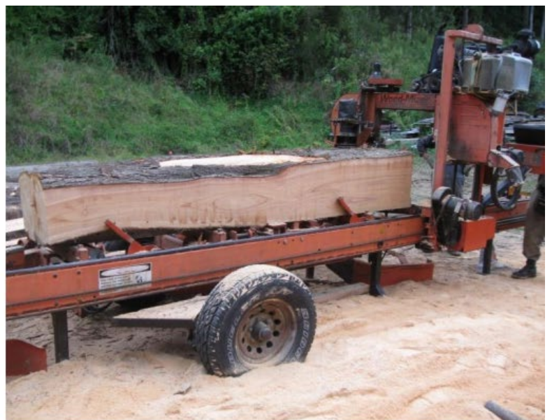
Left: A Wood-Mizer band sawmill in action quartering a pruned blackwood log. Right: A large pruned macrocarpa log being sawn with a Wood-Mizer. Photos: Paul Millen
