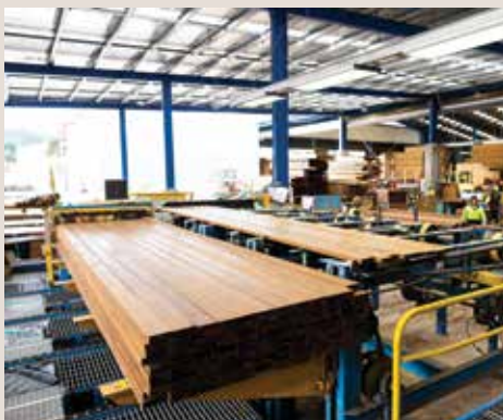
Thermal modification of New Zealand pine using heat and steam rather than chemicals enables it to have excellent thermal conductivity and natural durability and stability (source Abodo).
